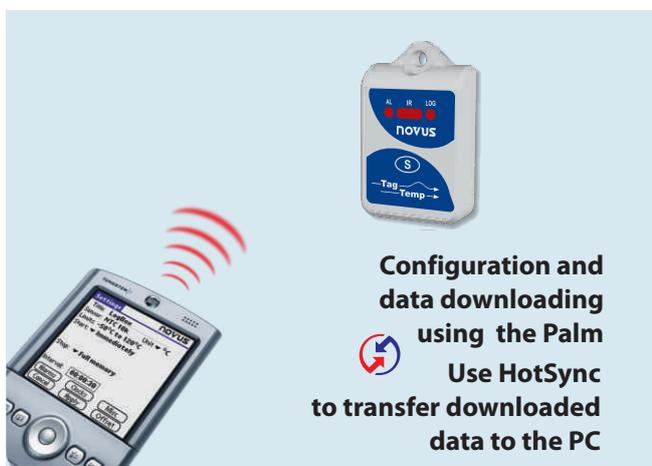
Configuring and downloading data with Palm OS compatible devices by means of the Infrared interface is easy and convenient. The data can be transferred to a PC through the HotSync synchronizer.
