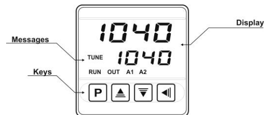
Fig. 02 - Identification of the parts referring to the front panel
