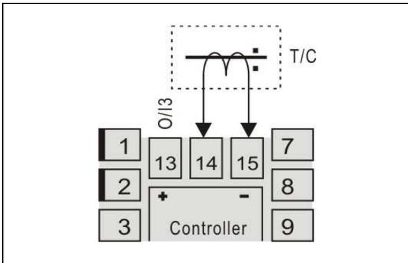
The CT was designed such as to facilitate its insertion in the load circuit. The CT core can be opened to allow the load wire to be installed inside the core, without opening the circuit. The CT wires may be stretched up to 3 meters long and must be kept away from other wires and cables of the installation.
