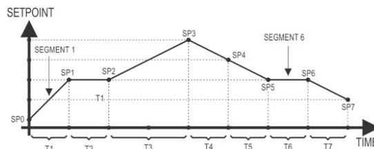
Fig. 04 - Example of a ramp and level program
