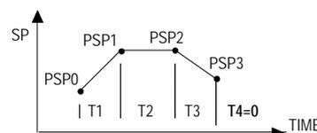
Fig. 05 - Example of a program with only 3 segments
