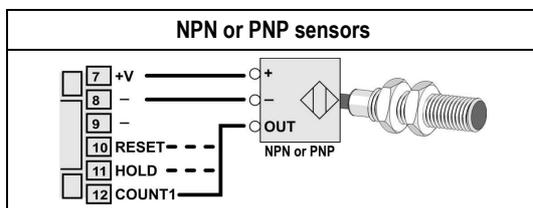
Figure 7a – Connections to the NC400-6 inputs
