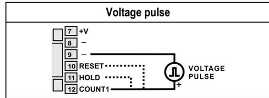
Figure 7c – Connections to the NC400-6 inputs
