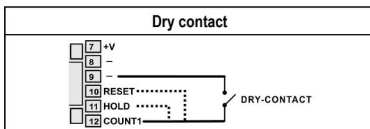
Figure 7b – Connections to the NC400-6 inputs
