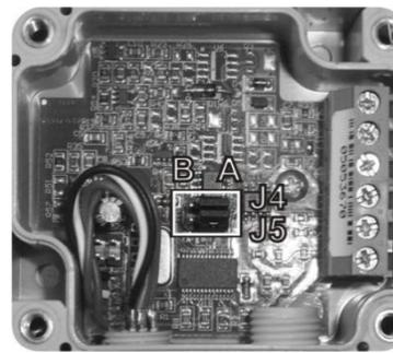
Figure 10 – J4 and J5 position within the transmitter
