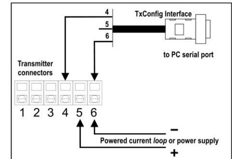
Figure 05 – TxConfig Interface connections – Loop powered
