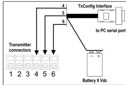
Figure 02 – TxConfig Interface connections model RS232.
