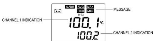
Figure 07 — SmartMeter display
