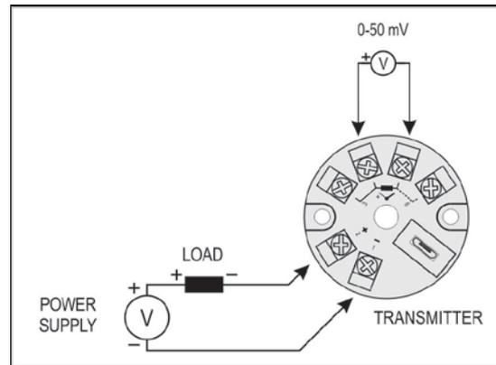
Fig. 9 – Transmitter electrical connections (0-50 mV)
