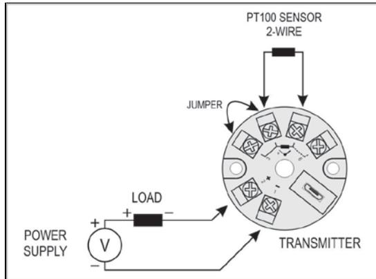
Fig. 5 – Transmitter electrical connections (Pt100 2-wires)
