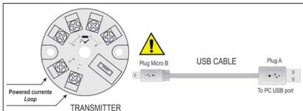
Fig. 2 – USB cable connections – Loop powered
