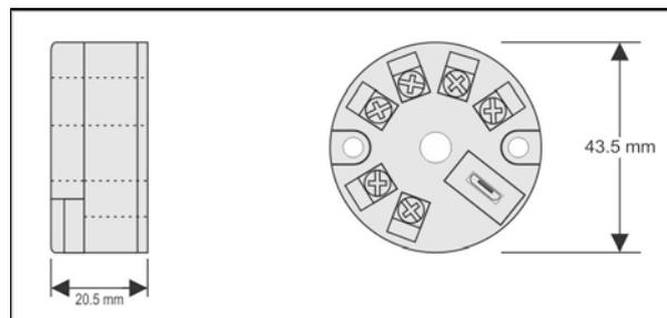
Fig. 4 – Transmitter dimensions
