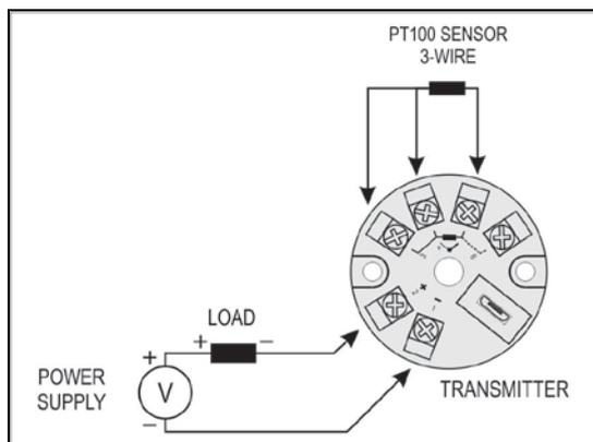
Fig. 6 – Transmitter electrical connections (Pt100 3-wires)
