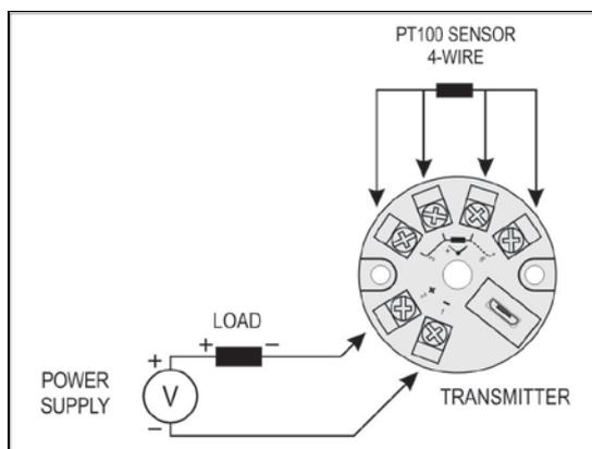
Fig. 7 – Transmitter electrical connections (Pt100 4-wires)
